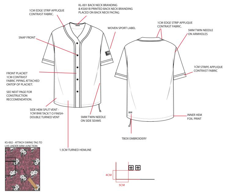
MEASUREMENT IS FOR T-BOX AND 4X4 POSITIONS
