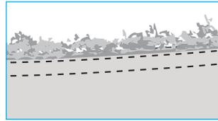
SEAM AT HOOD OPENING EDGE, BOTH LAYERS LEFT RAW. 2X PARALLEL STITCHLINE ALONG EDGE.
