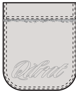
SELF FABRIC LHS CHEST POCKET APPLIED WITH TWIN PARALLEL STITCHING. EXTERNAL HEM AT TOP, WITH RAW EDGE. POCKET POSITIONED CENTRALLY TO FACING SEAM.
