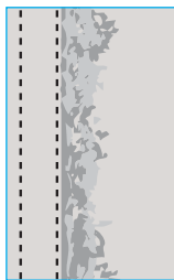
12CM WIDE EXTERNAL FACING AT CF. FACING IS MADE OF 2 LAYERS OF SELF FABRIC, FINISHED WITH 2 STITCHLINES AND RAW EDGE
