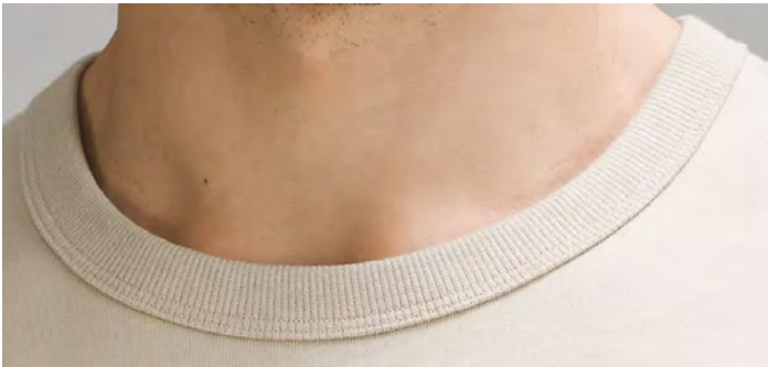
FOLLOW FOR NECK TRIM CONSTRUCTION - NECK RIB TOPSTITCHED ON BODY WITH DOUBLE NEEDLE
