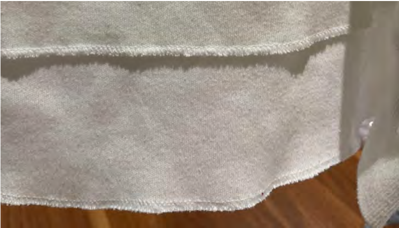
RAW HEM FINISHED WITH DTM SELF MERROW STITCH
