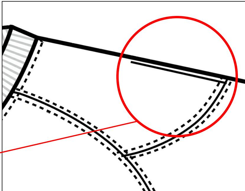
SHOULDER PANEL IS MISSING DART FOR SHAPING, PLEASE ENSURE THAT THIS IS ADDED. PLEASE ENSURE THIS DART IS USED FOR SHOULDER SHAPING, MEASUREMENTS CAN BE ADJUSTED AFTER SEEING NEXT SAMPLE
