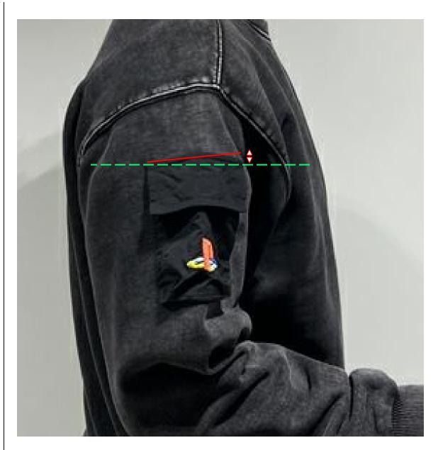
Sleeve pocket appears unbalanced and tilted, please ensure that the sleeve pocket sits evenly on sleeve when on body. To help this, please rebalance the sleeve and adjust the angle by approximately 3/8"
