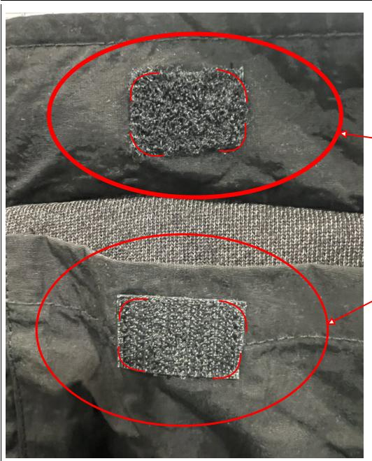
At the sleeve pocket, the velcro stripes exhibit sharp corners. It should be die-cut with round corners to avoid scratching when worn. Please improve this.
