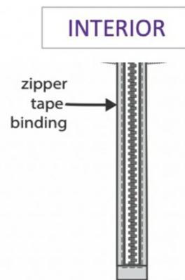
Detail of side slit construction
