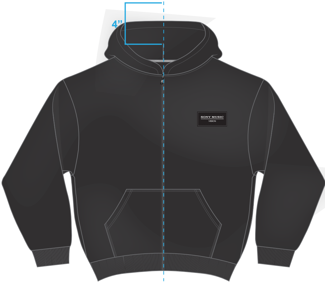
FRONT APPLIQUE = 2.5" WIDE PLACEMENT = 7.5" DOWN FROM HIGH POINT SHOULDER
